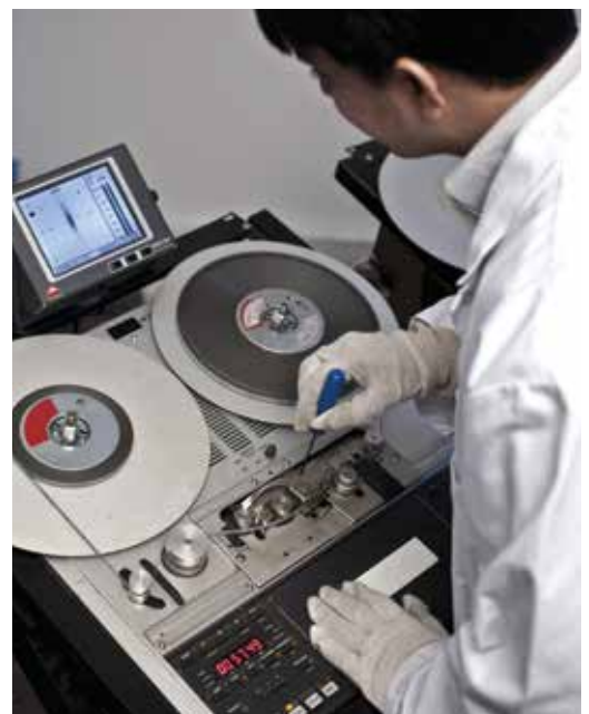
Azimuth adjustment on Studer A810
